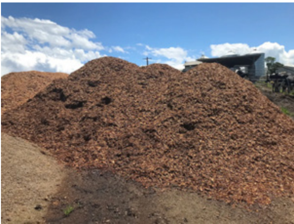
Shredded building waste.
