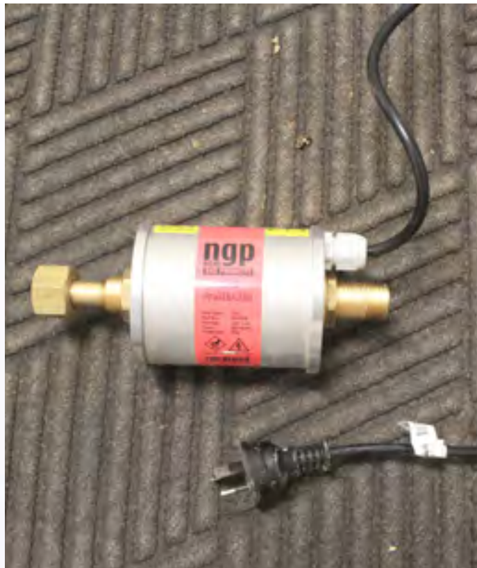
Photograph 10: CO 2 In-Line Heater Unit
