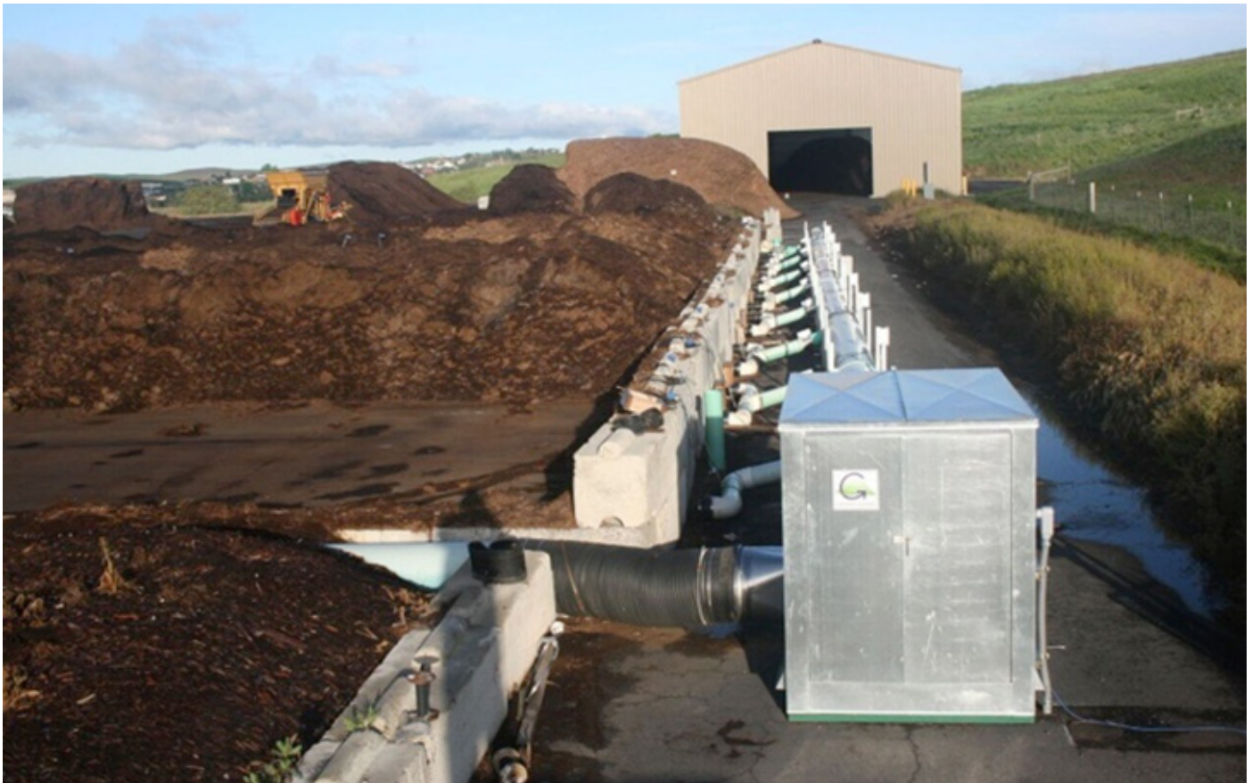
Figure 5: Forced aeration of a static pile
