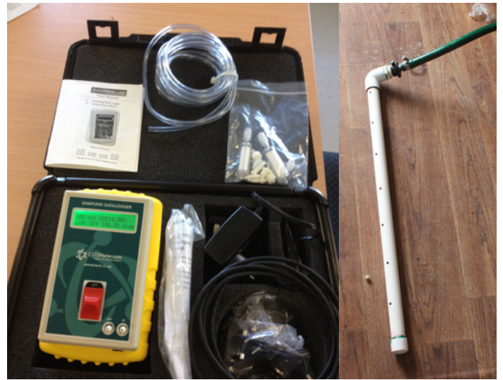
(L) Commercial CO 2 monitoring meter (R) Centralised gas delivery system
