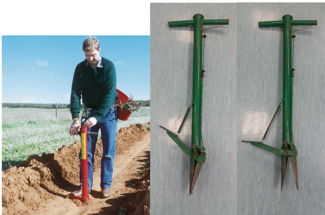
Figure 2. Left; PottiPutki planter in action. Middle; planter with beak mechanism in closed position ready for inserting into soil and Right; beak mechanism open ready for planting. The seedling is dropped down the hollow tube section of the planter and then the planter lifted up out of the way. Soil around the seedling is compacted by the operator's feet.
