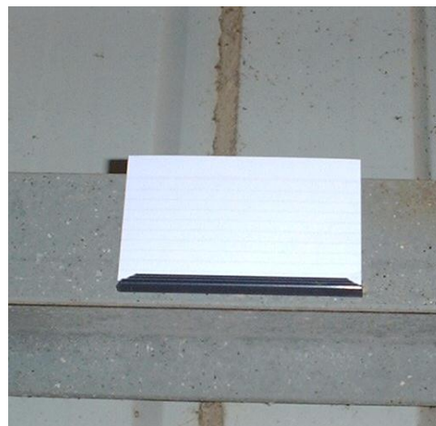
Figure 1: Spot card mounted on a support beam with a cut piece of poster holder for easy collection and replacement
