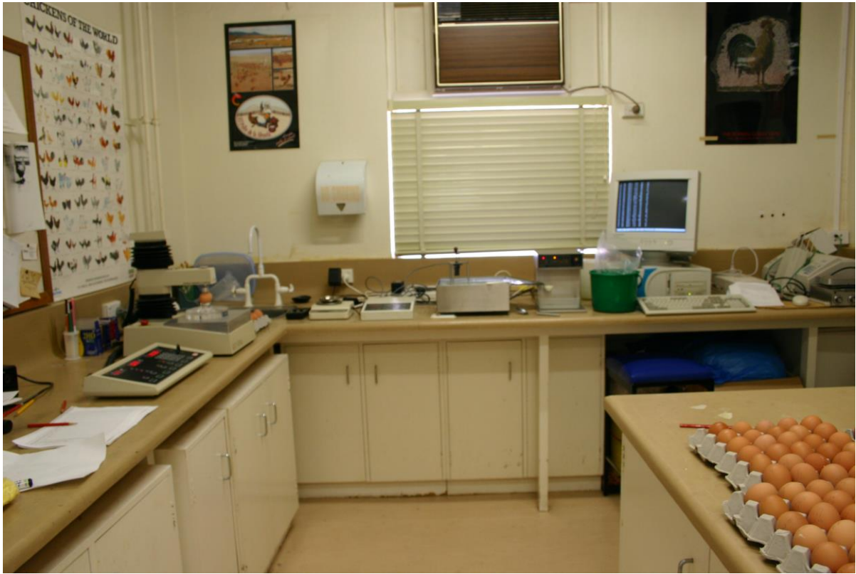
Photograph 2.3 The TSS equipment for measuring shell reflectivity and egg weight
