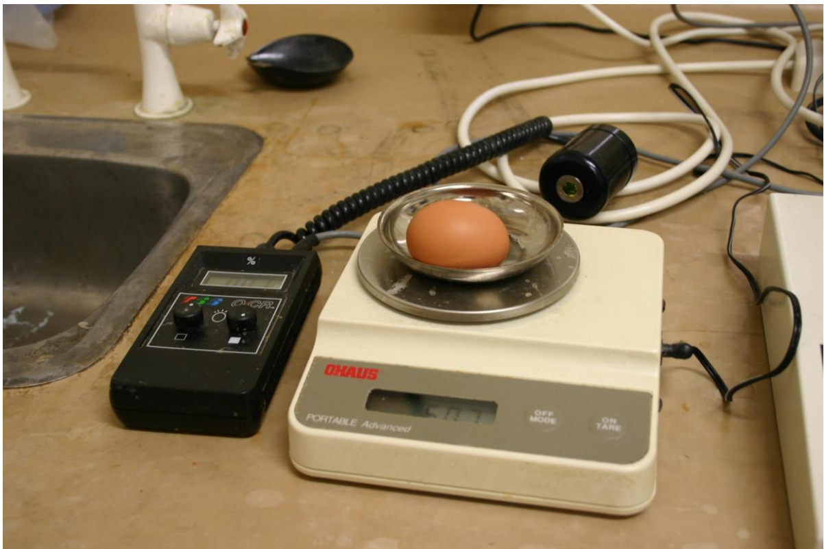
Photograph 2.3 The TSS equipment for measuring shell reflectivity and egg weight
