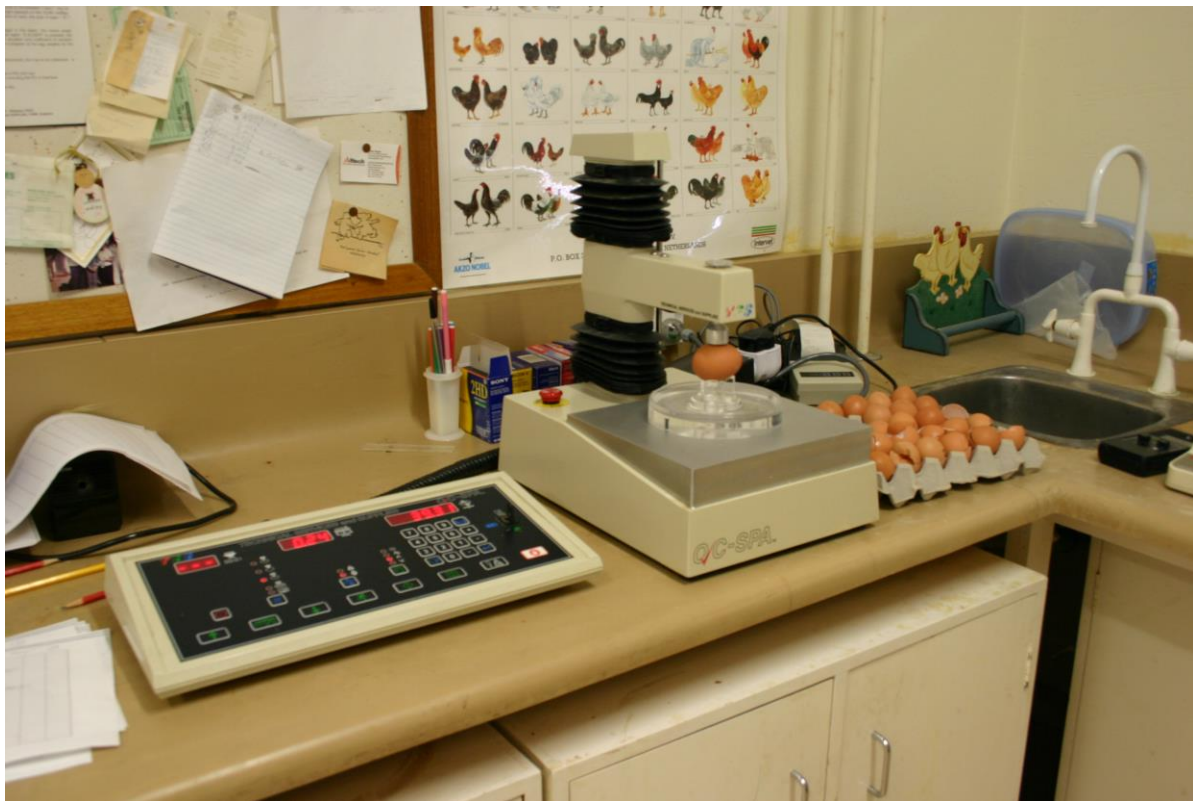
Photograph 2.5 TSS Equipment for measuring albumen height
