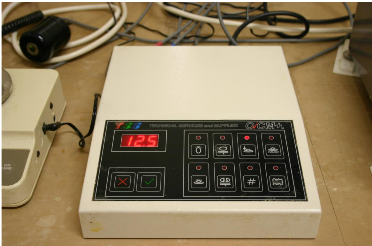
Photograph 2.7 The microprocessor that coordinates the input from the TSS equipment
