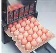
The ED SH Printer is designed for printing at higher speeds with one or two-line marking of eggs in grooved liners. The ED SH includes the EU printer with five printing heads. 5 rows of eggs are printed simultaneously, span 48 mm. The printer can be mounted on any transporters to carry the grooved liners at the speed of 15 to 40 cm per second.
