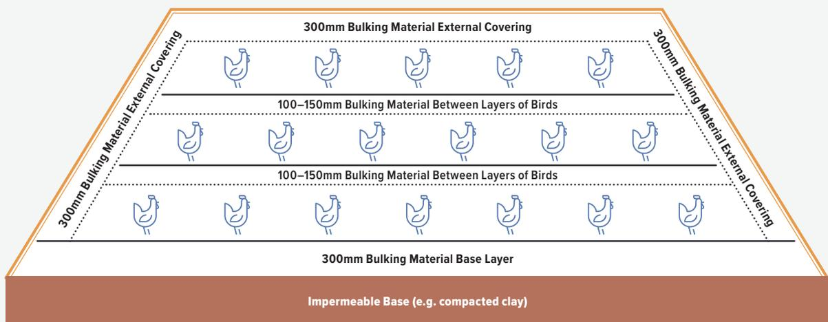
Figure 2. Carcass composting heap design
